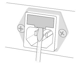
The fuse holder is an integral part of the IEC connector. It contains two fuses.
